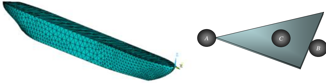
Figure 3. Constructions of the ship hull. a. Triangle elements and b. contact model.
